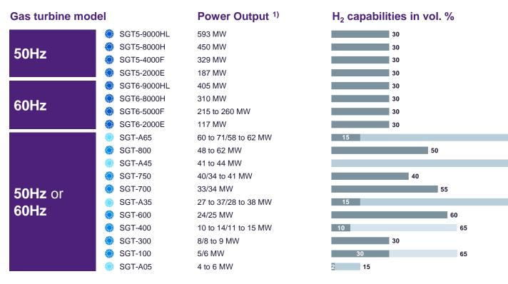
DLE burner WLE burner Diffusion burner with unabated NOx emissions Heavy-duty gas turbines Industrial gas turbines 1) ISO, Base Load, Natural Gas; Version 3.4, July 2020
